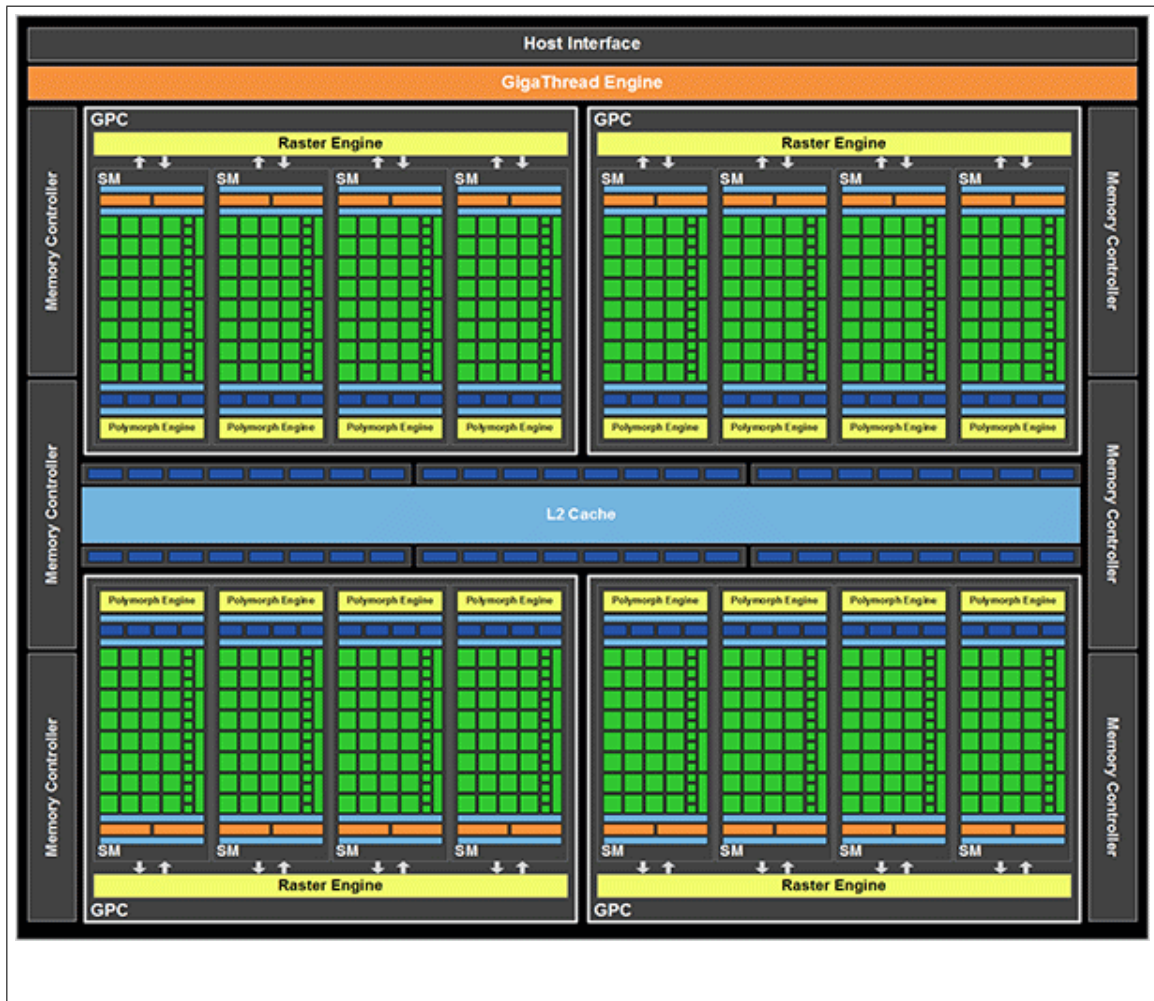
Figure 2.2: Kepler GF100 block diagram
